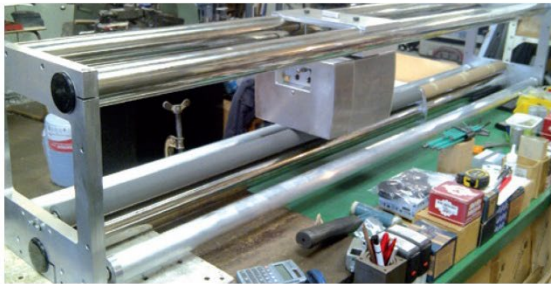
High strength bracket to resist deformation from high substrate tensions and for spans up to 2.11 metres
